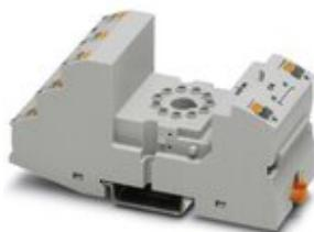
Relay base RIF-3..., for octal relays with 3 changeover contacts, Push-in connection, plug-in option for input/interference suppression modules, for mounting on NS 35/7,5
