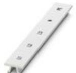
Zack marker strip, Strip, white, labeled, printed horizontally: L1, L2, L3, N, PE, mounting type: snap into tall marker groove, for terminal block width: 15.2 mm, lettering field size: 10.5 x 15.1 mm, Number of individual labels: 5
