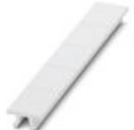
Zack marker strip, can be ordered: Strip, white, labeled according to customer specifications, mounting type: snap into tall marker groove, for terminal block width: 15.2 mm, lettering field size: 10.5 x 15.1 mm, Number of individual labels: 5
